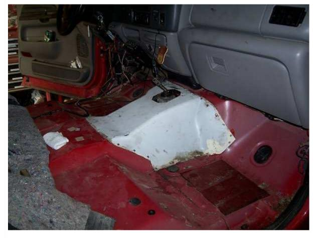
With the old floor hump out of the way there is LOTS of room to get to the tranny bolts. This is one reason i didn't bolt the floor hump back in place yet.
