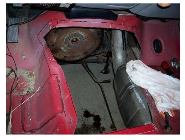
Now its time to install your new clutch. If you got your clutch kit from <u>South bend</u> it came with a new flywheel and everything you need. If not make sure you have the correct flywheel and I highly recommend putting in a new pilot barring at this time if it is a used flywheel. The one from <u>South Bend</u> already has a new one in it.
